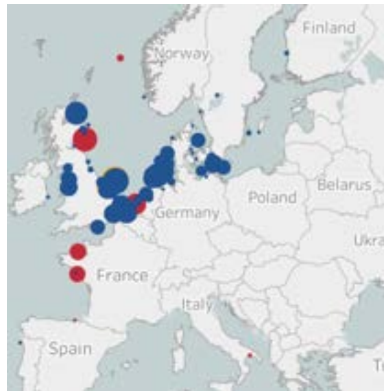
Figure 22: Offshore Wind Farms installed and under development in Western Europe 86
